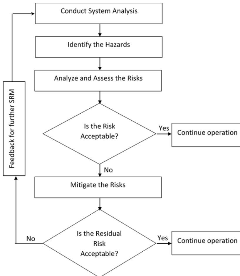
**Fig.1 SRM process flow chart**
